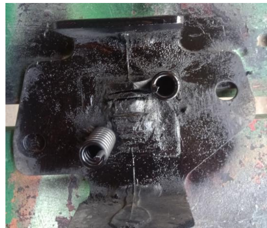
Gambar 2. Landasan mounting berbahan plat tebal 4 mm
